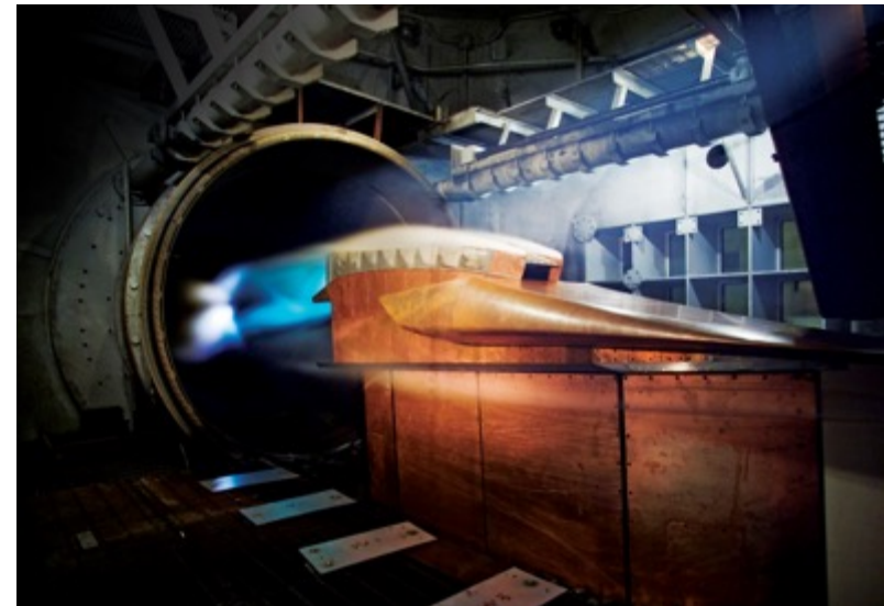
Hypersonic model in test chamber
