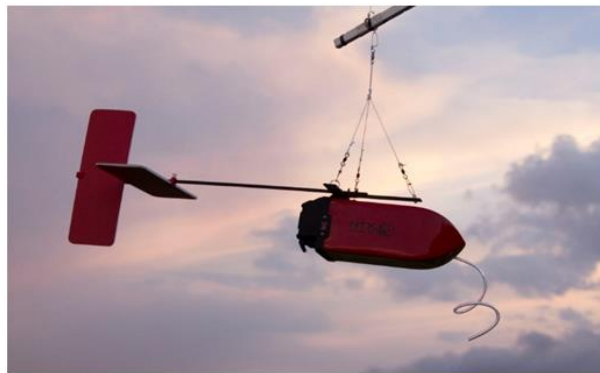
3 Figure 5. Schematic and picture of the miniGAS PRO, a 1.5kg miniature multiple gas payload 4 which incorporates waterproof case, GPS, SO 2 and CO 2 , temperature and relative humidity 5 sensors with onboard datalogger and telemetry, designed for UAV/ drone or tethered 6 balloon/blimp measurements.
