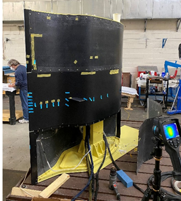
Component test concept for use in the Icing Research Tunnel at NASA Glenn Research Center.
