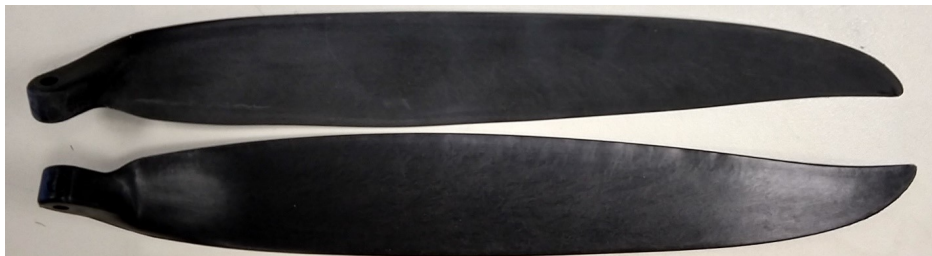
Figure 4. Comparison of the custom CCW rotating (upper) and COTS CW rotating (lower) propeller blade planforms, as viewed from the bottom.
