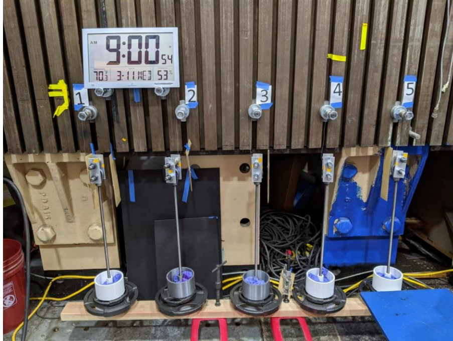
Figure 9. Conventional test stand final set-up, loading 5 specimens.
