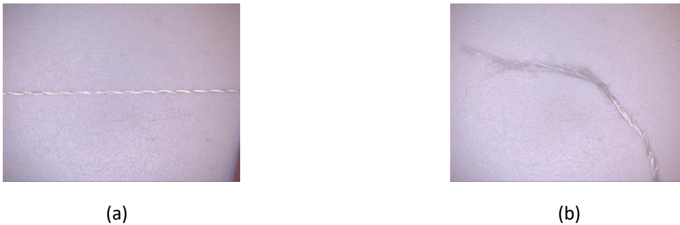
Figure 1. Pictures of (a) pristine and (b) failed Vectran yarn taken via a USB microscope.
