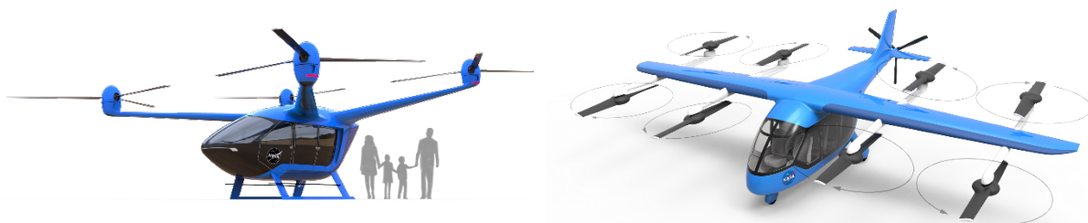
Figure 1: NASA RVLT reference vehicle configurations considered in this study: quadrotor (left) and lift plus cruise (right).
