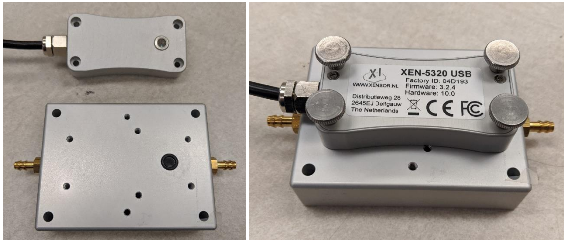
Figure 3. XEN-5320 sensor and manifold disassembled (left) and configured for testing (right).
