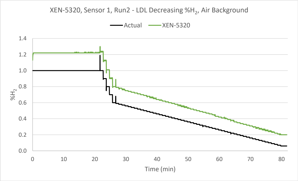
Figure 84. XEN-5320 data for sensor 1, run 2 of the LDL test with decreasing %H 2 in an air background.
