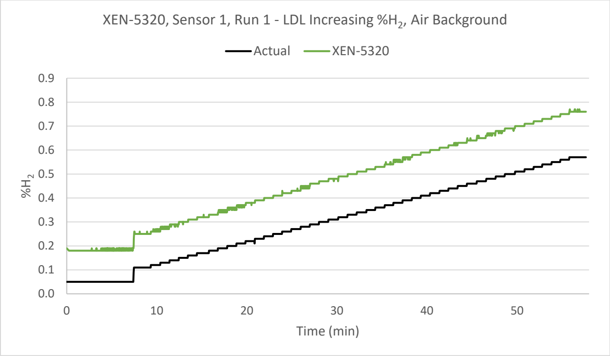
Figure 67. XEN-5320 data for sensor 1, run 1 of the LDL test with increasing %H 2 in an air background.
