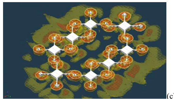
Figure 22. One Possible Modular Rotorcraft Configuration: (a) single vehicle 'element,' (b) swarm of small independent rotorcraft 'elements,' and (c) vehicle 'elements' integrated into a modular rotorcraft configuration
