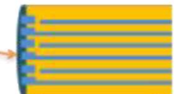
Arc Sprayed Termination
