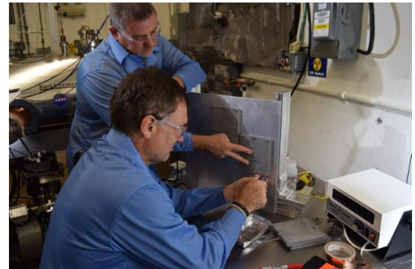
Preparing sample plate with live propellant
