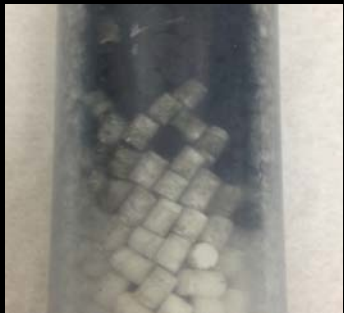
Sabatier catalyst material after vibration testing
