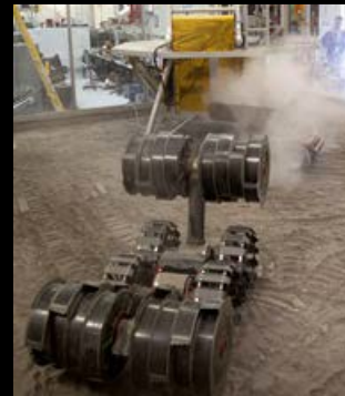
RASSOR excavator delivering regolith
