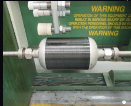
Filament Winding of Composite Overwrap Pressure Vessel (COPV)
