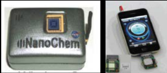
(L) CNT "Electronic Nose"; (R) Nanochemsensor flown on ISS
