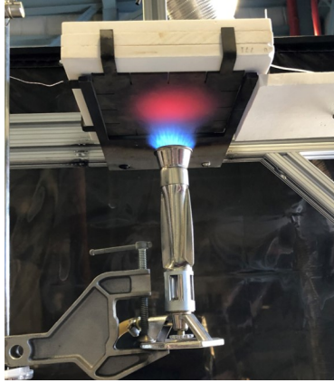
Figure 2: THERMIC setup with Meker burner during a test.
