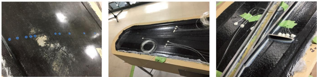
Figure 16. (left) External view of the three-dimensional printed flush pressure ports (row 4); (center) internal view of the three-dimensional printed flush pressure ports (row 4); and (right) internal view of the flush port installed in the elevon control surface with tubes attached.
