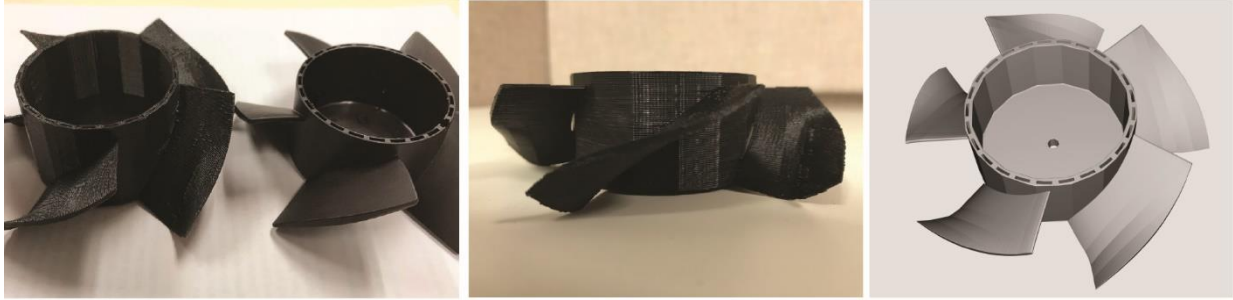
Figure 24. Fan assembly: (left) a new fan blade assembly; (center) the original fan assembly; and (right) new fan blade assembly 3D print graphic.
