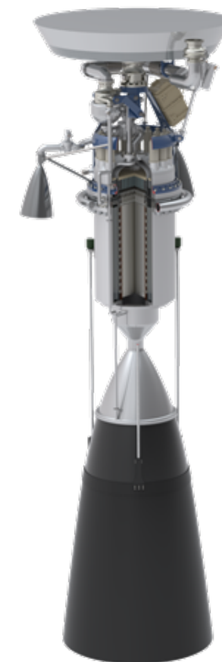
NASA's Nuclear Thermal Propulsion Engine System (GCD – 875 sec Isp, 25,000 lb f ) is shown, of which BWXT and Aerojet Rocketdyne are providing support for engine, reactor and fuel design and analysis.
