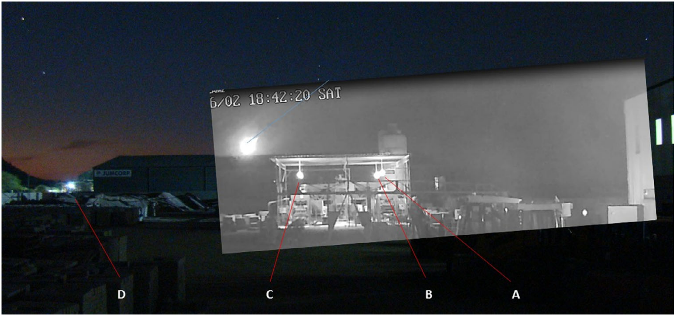
Fig. 8. Gaborone meteor video frame (gray) on top of calibration image (color). Letters refer to Table 3.
