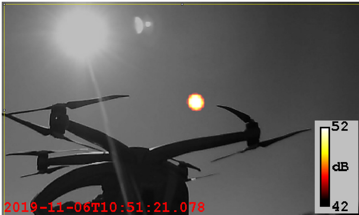
Figure 15.—Phased array beamforming image for 55 percent motor speed, left rear top rotor, 1208 Hz.
