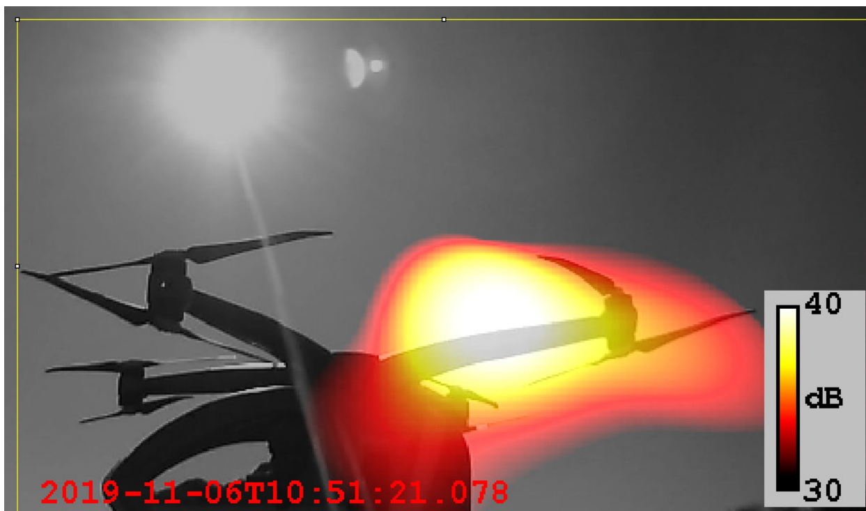
Figure 16.—Phased array beamforming image for 55 percent motor speed, left rear top rotor, 4585 Hz.
