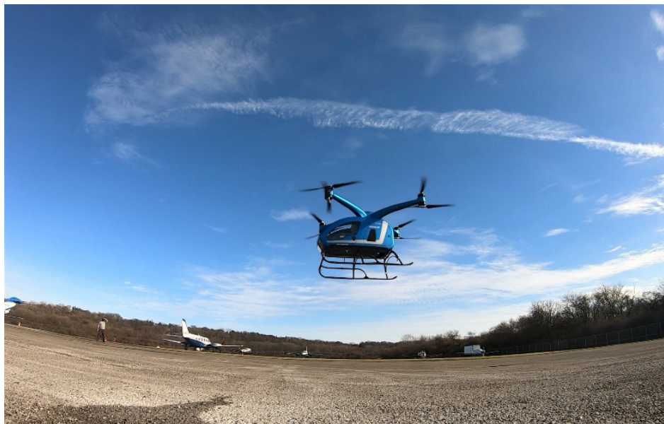
Figure 1.—Moog, Inc. SureFly proof-of-concept all-electric research vehicle.
