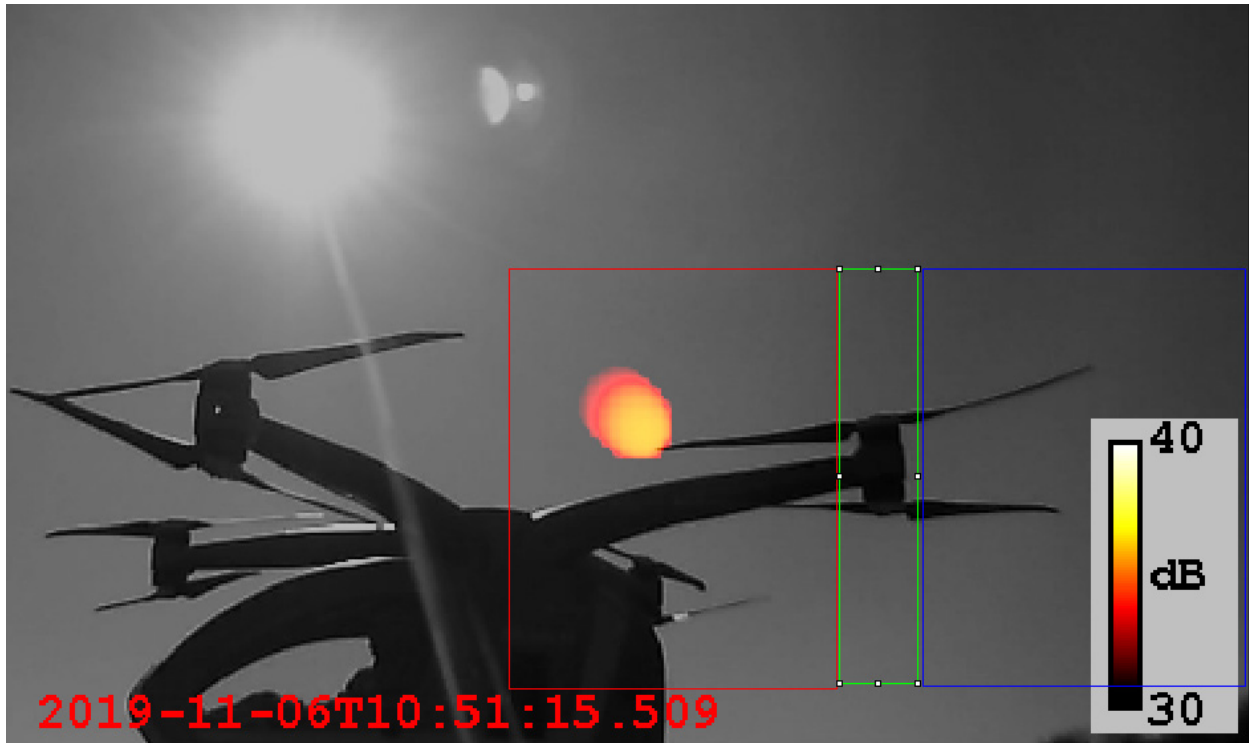
Figure 17.—Partitions for source separation, red box for advancing blade, green box for hub/motor region, blue box for retreating blade. Phased array beamforming image for 55 percent motor speed, left rear top rotor, 4585 Hz.
