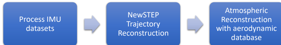
Figure 6: MER Reconstruction Process
