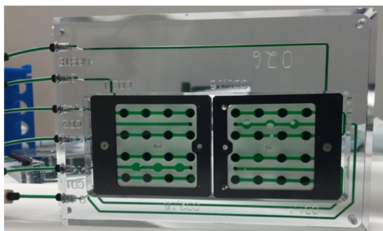
Figure 6. Well Plate Adapter (right) with incorporated fluidic cards. Embedded fluidic channels filled with green dye for visualization. Surrogate manifold schematic (left) featuring standard lab fluidic components.
