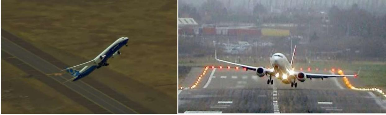
*Figure 1. Images demonstrating the type of maneuvers that are required for Part 25 certification: (left) High alpha demonstration and (right) crosswind takeoff.*
