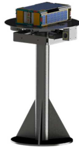
Air bearing at JPL's Small Satellite Dynamics Testbed with mock satellite
