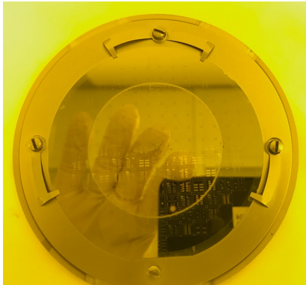
75 mm Diameter Gen. 11 Wafer Just After Metal1 Deposition
