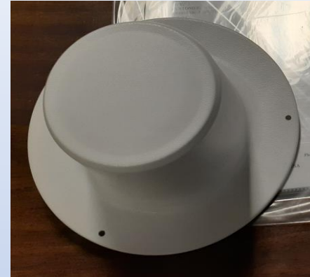
Omnidirectional antenna Electro-Metrics 6853 installed on the van, ultra-wideband (300 MHz-40 GHz), 2.82 m above ground level
