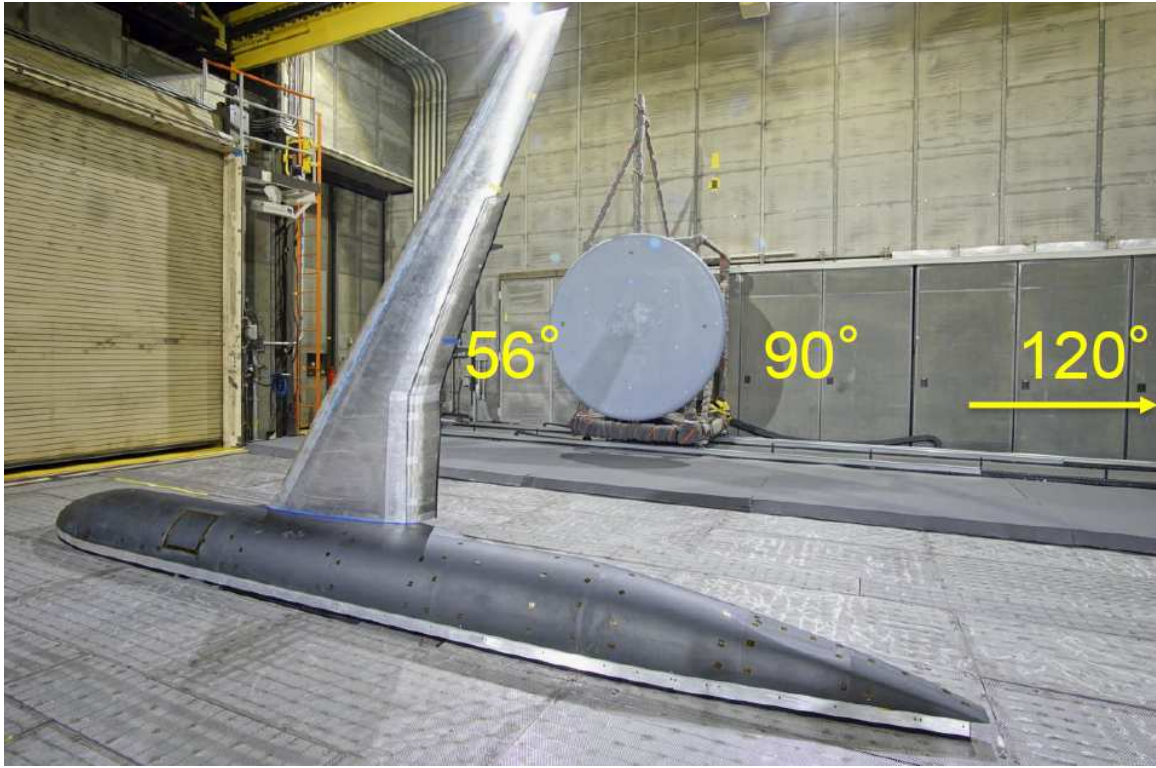
Fig. 11 Photo of the microphone array at 70°. The 90° position is directly below the model, in line with the center of the balance. Approximate array positions are also indicated.
