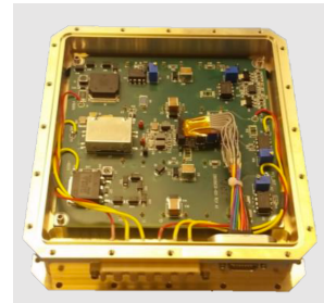
High Voltage Driver
