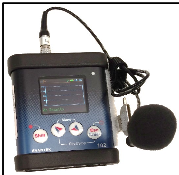
Figure 1. Svanetek SV 102A+ Class 1 Dual-Channel Noise Dosimeter, a.k.a. Acoustic Monitor.
