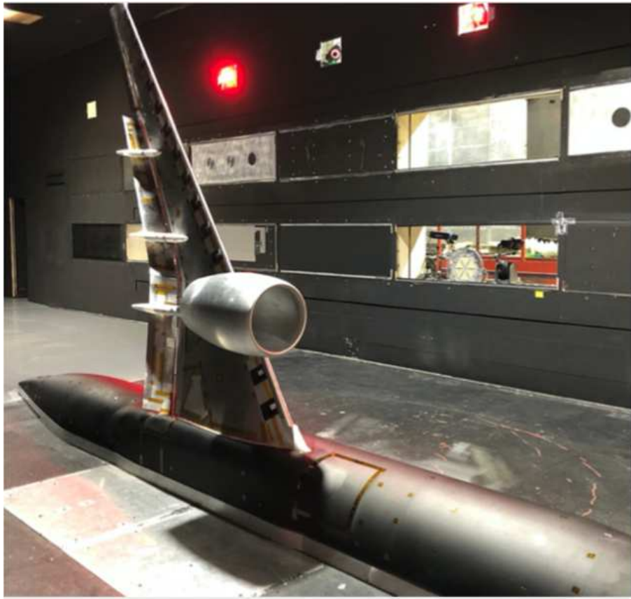
Fig. 1 Global view of the conventional high-lift CRM configuration in the 14x22 wind tunnel.
