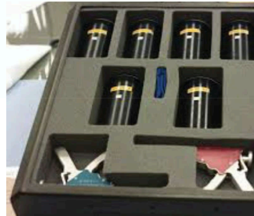
Fig. 3 BRIC-60 Canisters as flown
