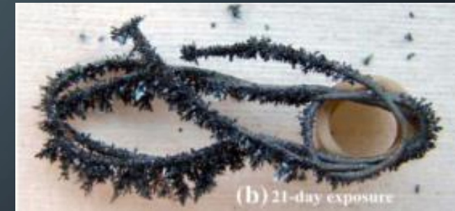
Reactivity Example: 21 day exposure of nickel clad copper wire (Lukco et al, 2018 to Venus surface atmosphere in the NASA Glenn Extreme Environment Rig (GEER)) https://agupubs.onlinelibrary.wiley.com/doi/pdf/10.1029/2017EA000355
