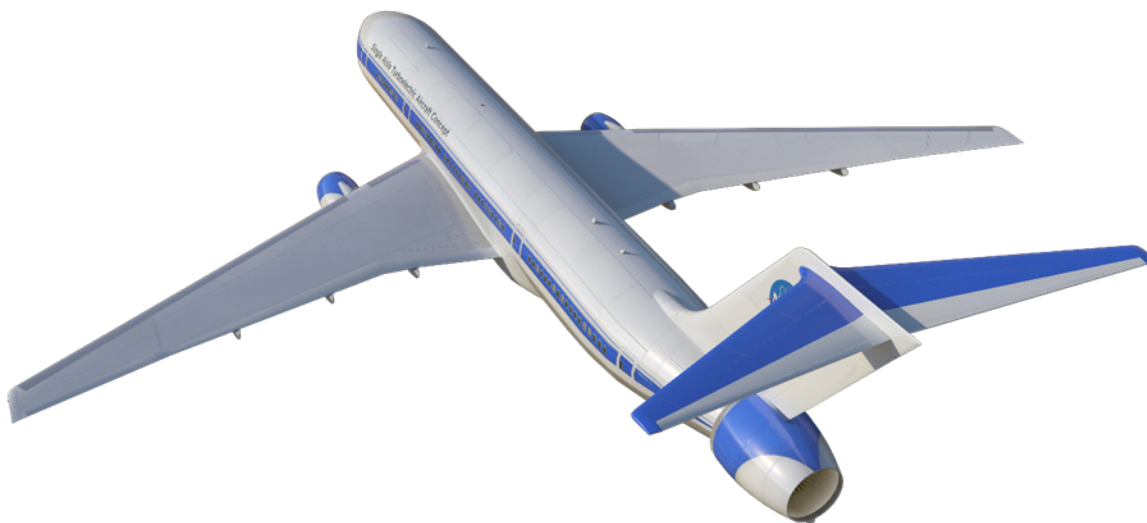
Figure 7.—Artist conception of single-aisle turboelectric aircraft with aft boundary layer propulsion (STARC-ABL) showing integration of boundary layer ingestion propulsor and T-tail.
