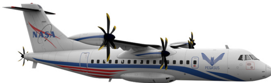
Figure 4.—Hybrid-electric Parallel Electric-Gas Architecture With Synergistic Utilization Scheme (PEGASUS) concept.
