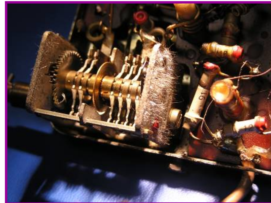
Tin Whiskers on 1960's Era Variable Air Capacitor
