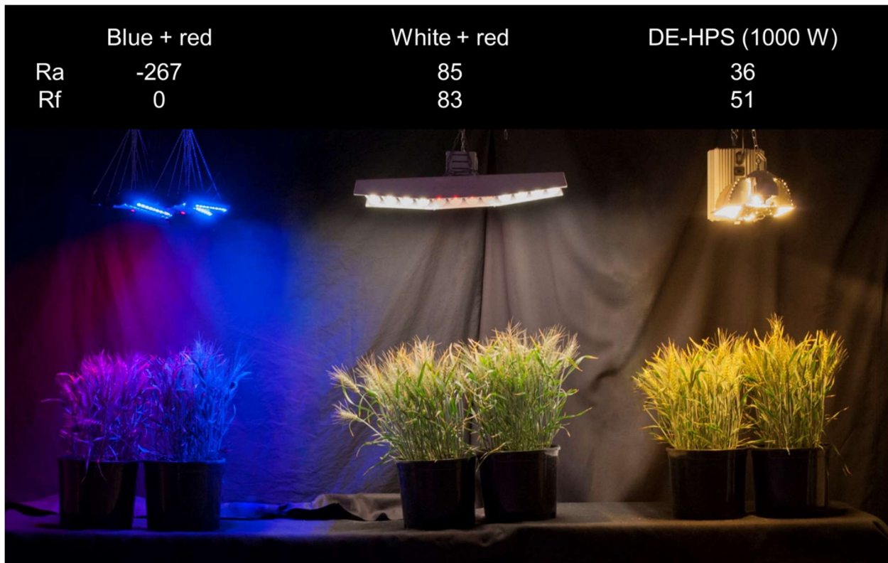
Figure 7. Visual quality of wheat growing under a blue + red combination of LEDs (left), a white + red combination of LEDs (middle), and a double-ended high-pressure sodium lamp (DE-HPS; right). Calculated CIE color rendering index (CRI Ra) and TM-30-18 color fidelity index (Rf) are provided for each light source. The photon intensity under the light sources was uniform.
