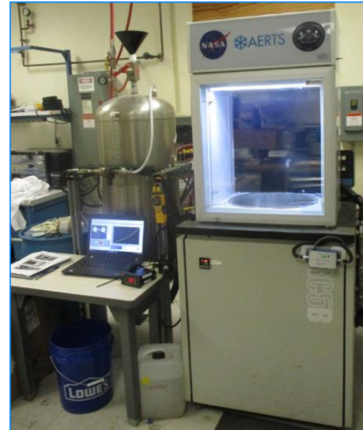
AERTS Jr. (Adverse Environment Rotary Test Stand) based on larger instrument at PSU, POC; Dr. Jose Palacios
