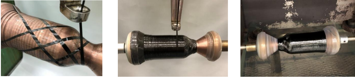
Figures 2-4. 2k Filament Winding Process
