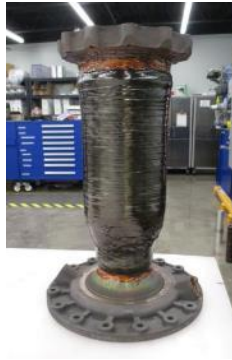
Figure 20. Final Composite Overwrap Chamber Post Cure
