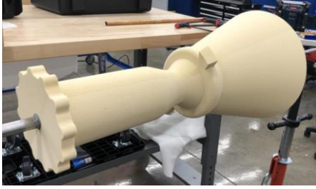
Figure 9. High Temperature Foam Mandrel
