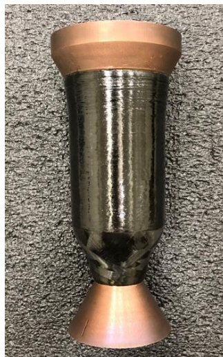
Figure 5. Final 2k Chamber Post Cure
