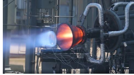
Figures 21-22. February 7k Hot fire Test
