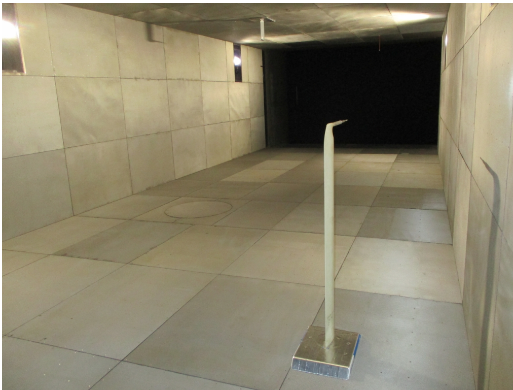
Fig. 5 Experimental setup for background noise validation measurements in test section.
