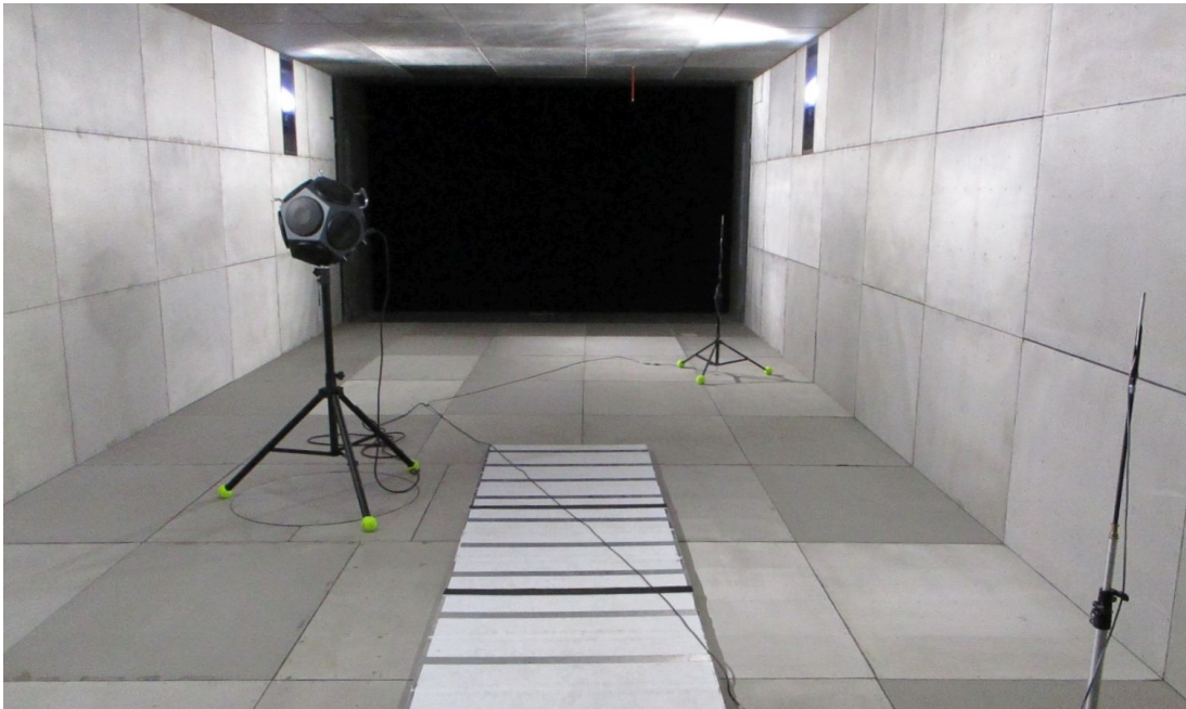
Fig. 7 Dodecahedron speaker in the 9x15 LSWT test section at the location of a typical fan model. Test conducted June 27-18, 2019. Looking upstream from diffuser ramp.
