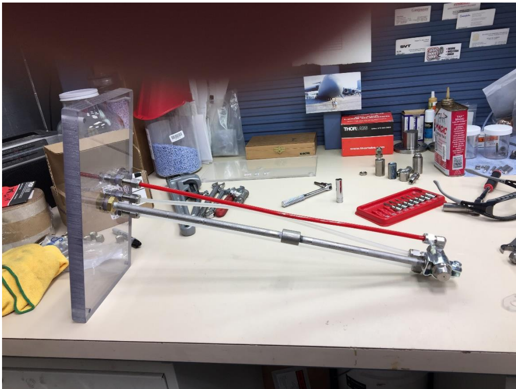
Fig.7 Rod supporting the Nozzle and Window supporting the Rod, and Two Connectors for Air and Water Supply
