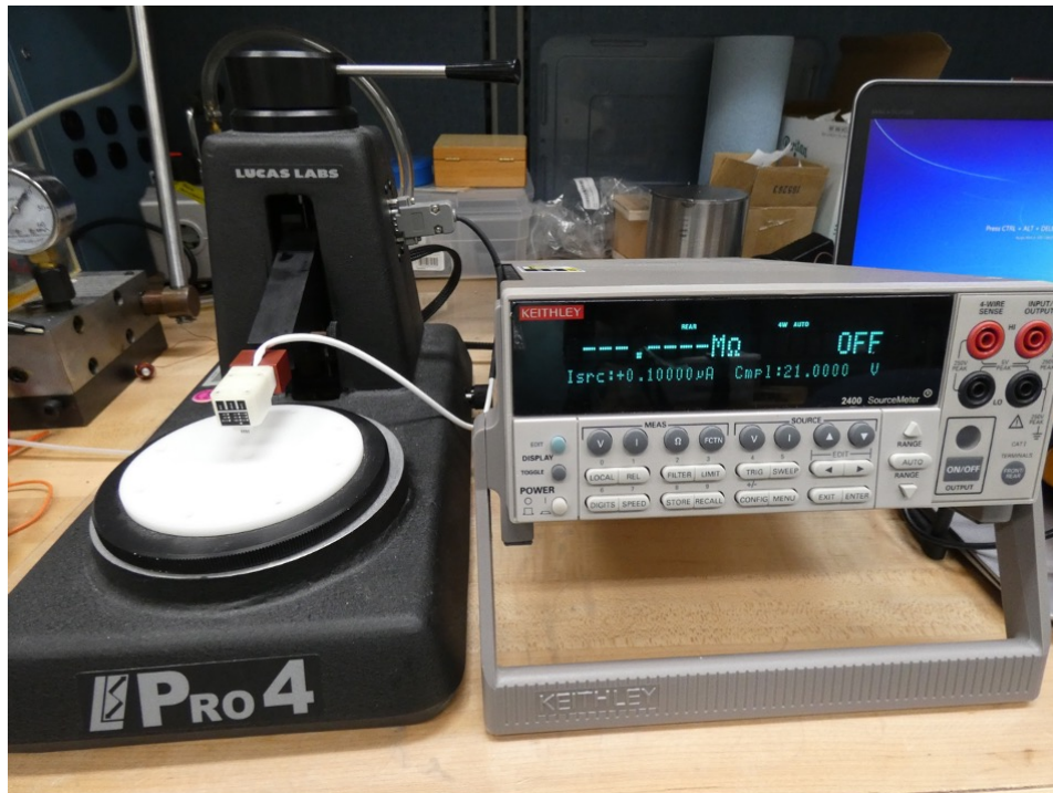
Figure 11. Photo showing the four-point system used to measure the resistivity of the charred AVCOAT at room temperature.
