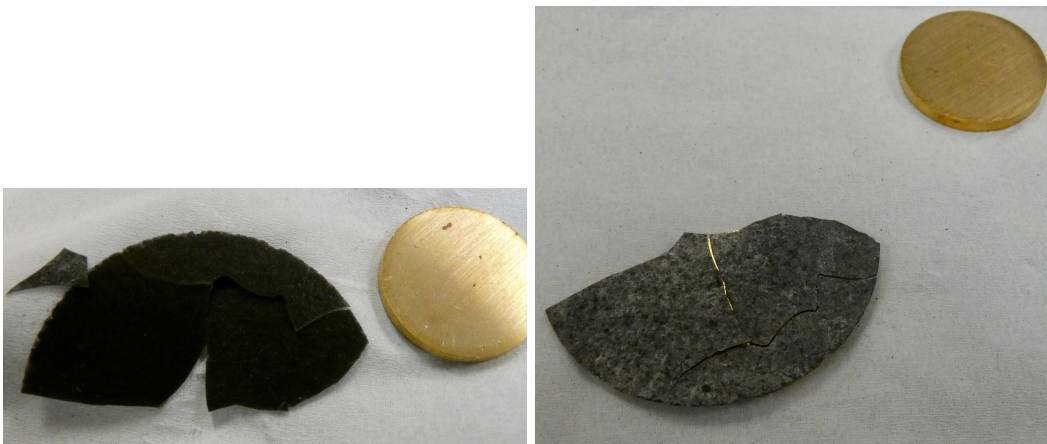
Figure 42. Photos showing both sides of the outer coating taken from an AETB tile. The outer surface is on the left. The inner surface (right) still show some of the white coloration of the insulating glass fibers. This sample when whole is 40 mm in diameter and 0.36 mm thick. 20 mm electrodes shown in the photos where used to test the sample fragment shown.
