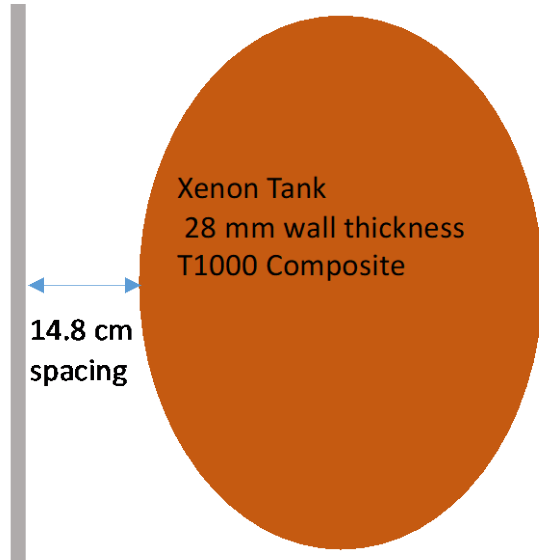
Figure 6-18 Illustration of the Initial Xenon Tank and Bulkhead
