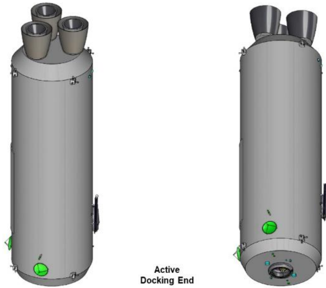
Figure 3-16 Stowed Configuration of the Chemical Propulsion Module
