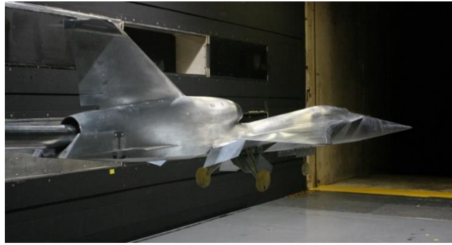
Fig. 6 GLBC model with flaps deflected 30^\circ and landing gear deployed (landing condition) configured for OGE testing in the LaRC 14x22 tunnel.
