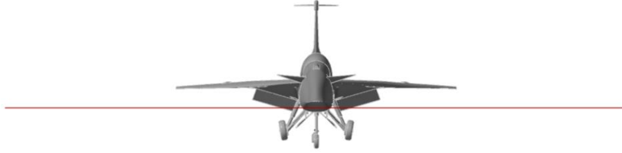
Fig. 24 Extent and position of beamforming plane. Grid resolution: 0.02 m.
