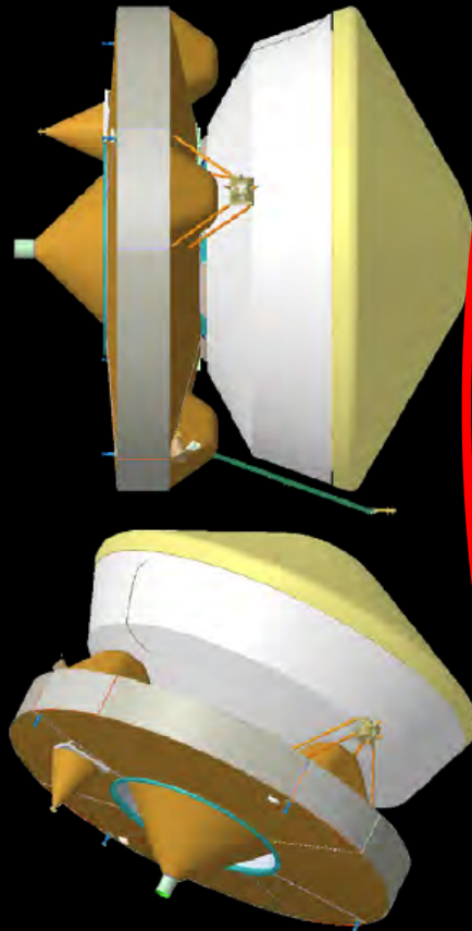
Spacecraft = Cruise Stage + Entry Vehicle
