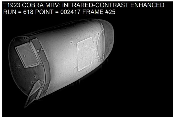
**Fig. 9 Infra-red image of the model surface showing transition occurring at or before the grit elements. Mach number 3.48, Re 3 M/ft.**
