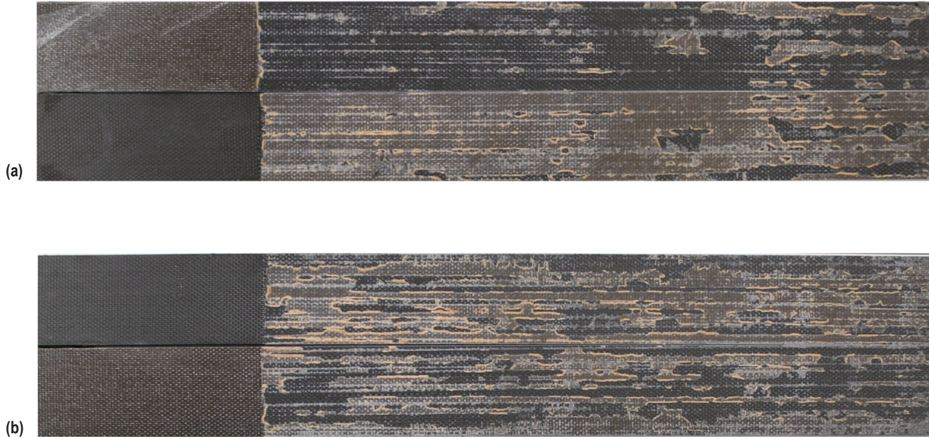
Figure 15. Representative fracture surfaces from 200 °F cure temperature test groups with extended adhesive out-time (40 days): (a) without APPT and (b) with APPT.
