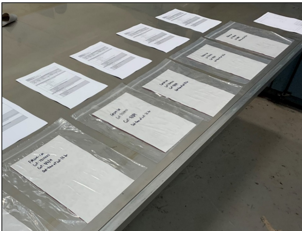
Figure 6. Film adhesive for extended adhesive out-time groups during aging period in NASA MSFC composites fabrication facility.
