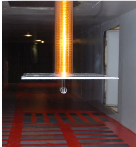
Fig. 7. Common Reference LWC probe, the SEA MW, installed in the IRT.
