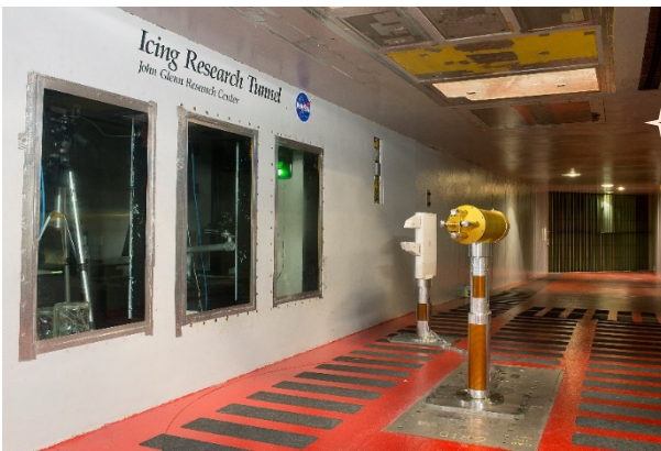
Fig. 9 IRT primary (P) location and secondary (S) locations. Primary is at tunnel center (0, 0, 36): a) sketch of IRT test section showing the Secondary (S) floor mount placement at (69, 30, 0); probes in the secondary position (S) were typically 24-in from the floor; b) image with 2D-S at Primary location, and HSI-FPDR at Secondary location; c) Image showing PSI-FPDR-2 in Primary location and ceiling-mounted MW in aft secondary location at approximately (48, 24, 36).
