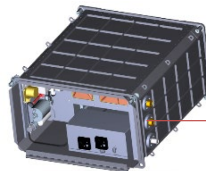
Far Field Diagnostics (in Mid Deck Locker) Avionics, CO 2 scrubber, Smoke Eater, Combustion Products Monitor, particulate monitors (DustTrack & Ion Chamber)
