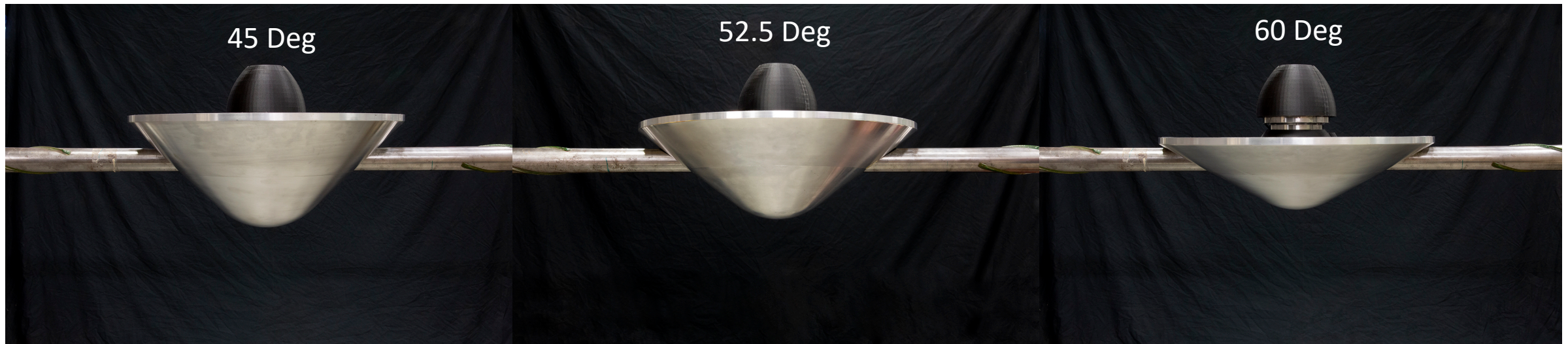
Boeing CST-100 (Abort Configuration) - December 2014 Prior test in TDT that used Transverse Sting and OTT
