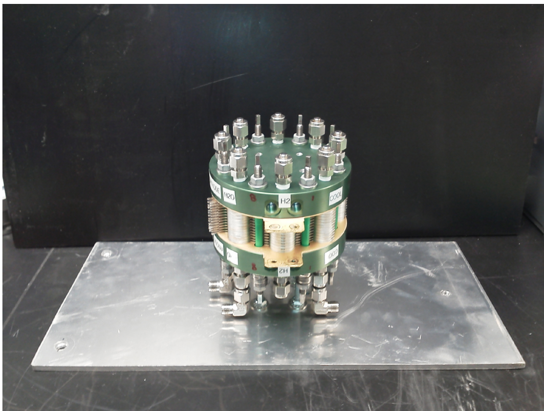
Figure 3.—Twelve-cell proton exchange membrane (PEM) fuel cell stack.
