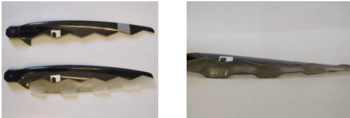
(a) KDE Blade with Trailing Edge Cuts (Top) and Completed Trailing Edge Modified Blade (Bottom) (b) Front View of Completed Trailing Edge Modified Blade
