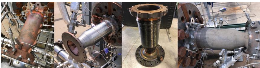
Fig. 9 7k lbf chamber liner configuration from left to right: LLAMA, ALPACA, COMET, META4X4
