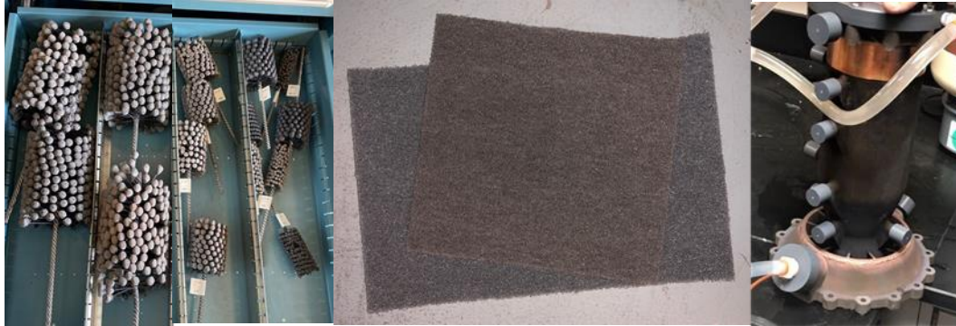
Fig. 15 Honing bits used on all chamber liner hardware thrust classes (left), Scotch Brite abrasive pads (middle), and chemical mechanical polishing setup (right).
