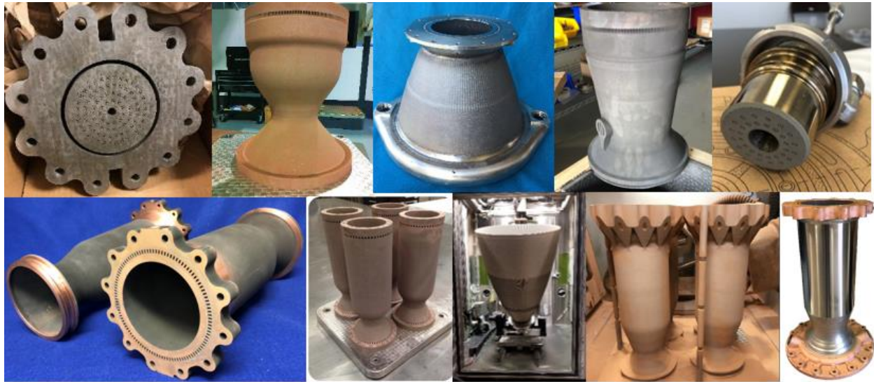
Fig. 1 Images of various combustion device hardware that utilize L-PBF and LP-DED techniques.
