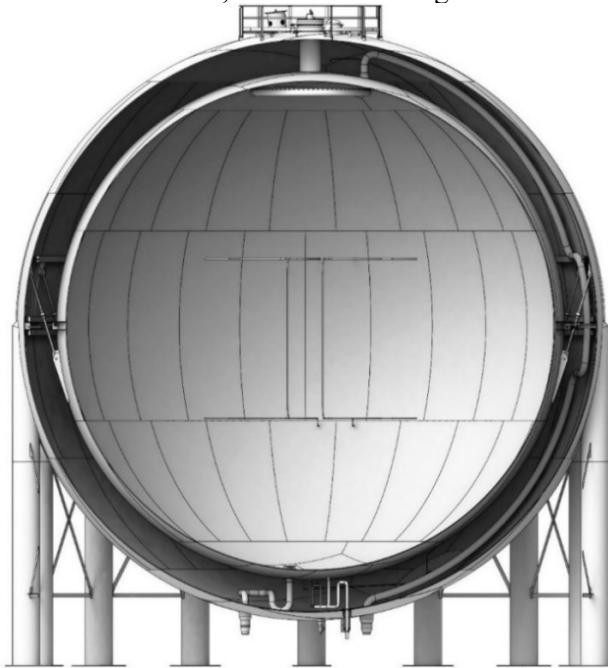
Figure 2. Overall elevation view of the new 4,700-m 3 LH 2 storage tank.
