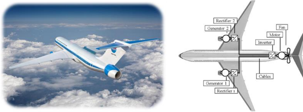
Figure 1. STARC-ABL Conceptual Design and the Notional Power System
