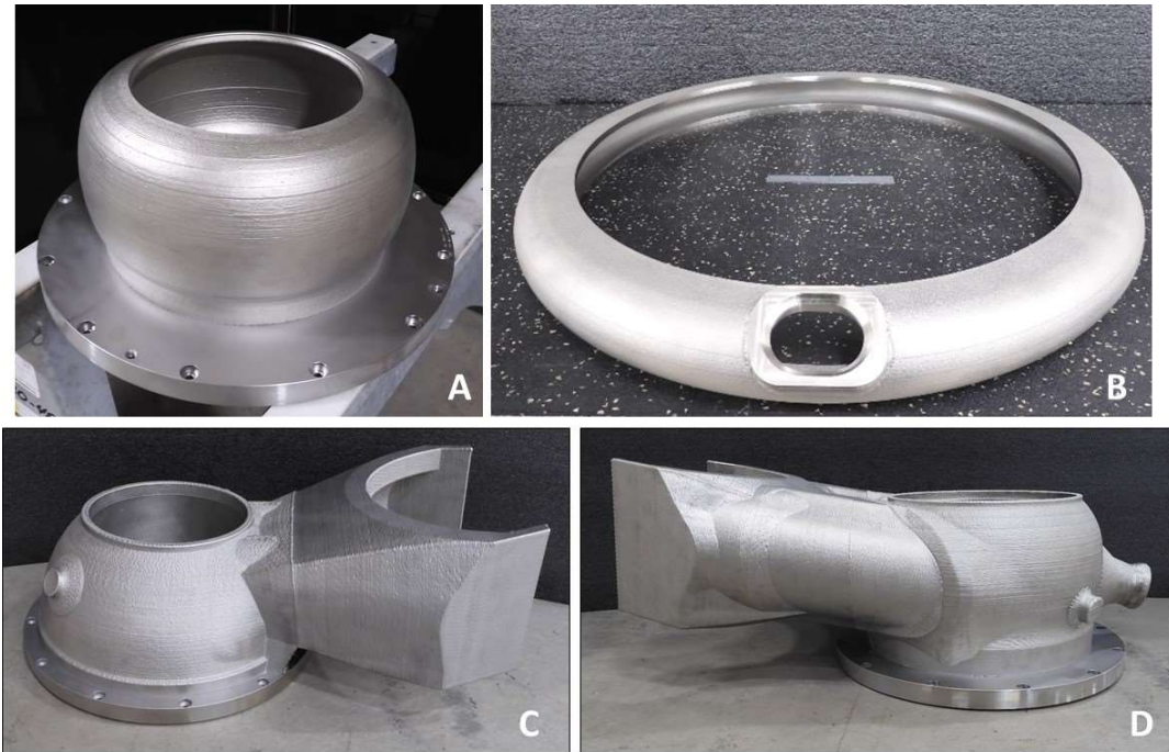
Figure 11. Examples of thick-wall LP-DED hardware. A) Liner for powerhead, B) 24" dia. manifold for subscale nozzle, c) RS-25 hot gas manifold oxidizer shell, D) RS-25 hot gas manifold fuel shell.
