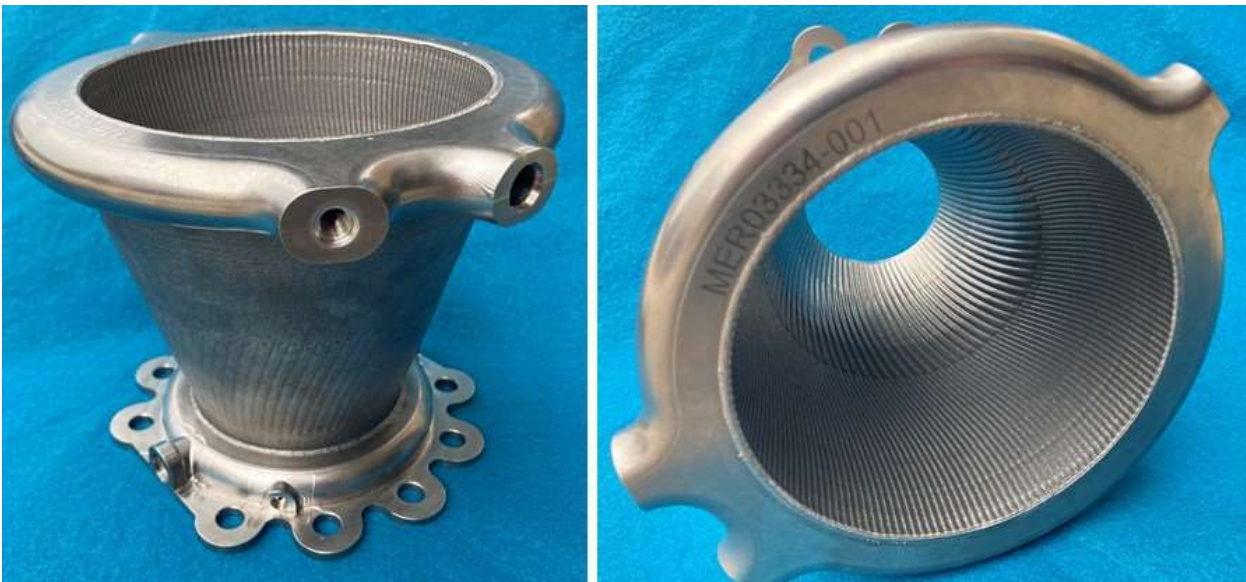
Figure 14. 1.2K- lb f integral channel LP-DED scalloped spiral nozzle hot-wall after CMP processing.
