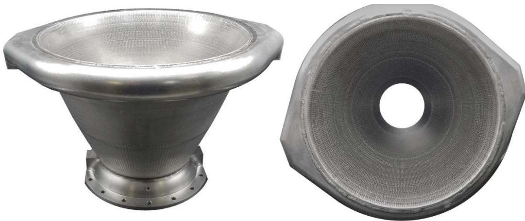
Figure 17. Post chemical mechanical polishing (CMP) of the hot wall for improved surface finish and reduced total heat load performance.
