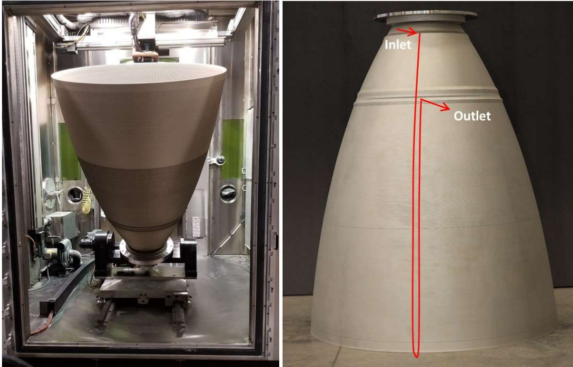
Figure 12. NASA HR-1 65% scale integrated channel wall nozzle fabrication using LP-DED built in 90 days [Diameter = 58 inches (1.47 meters) and the total height was 72 inches (1.83 meters)].
