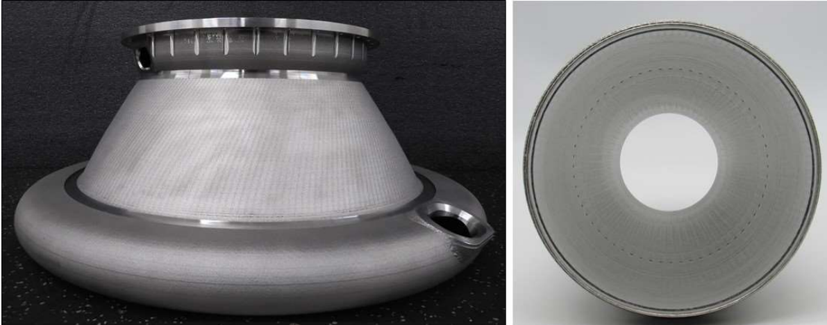
Figure 13. NASA HR-1 Nozzles fabricated using LP-DED process. (Left) 40K- lb f nozzle with spiral channels with manifolds fitted prior to EB welding, (Right) 1.2K- lb f nozzle hot-wall after CMP processing.
