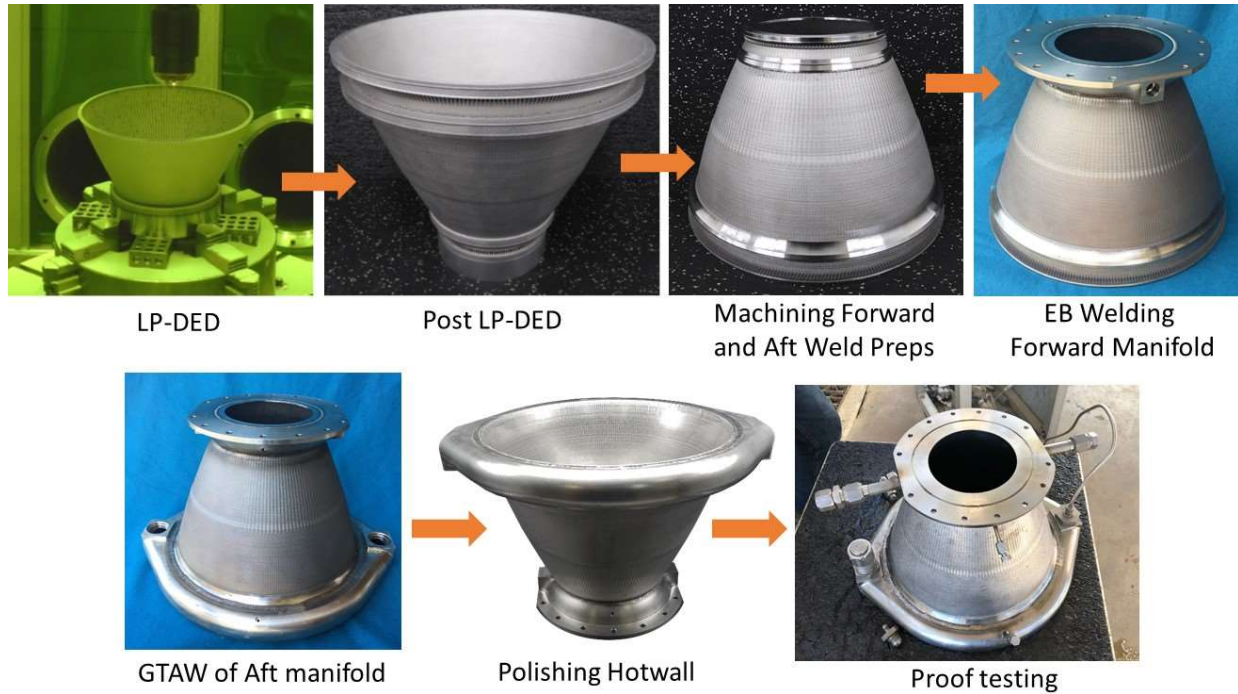
Figure 16. Visual process flow and progression of hardware leading into hot-fire testing.
